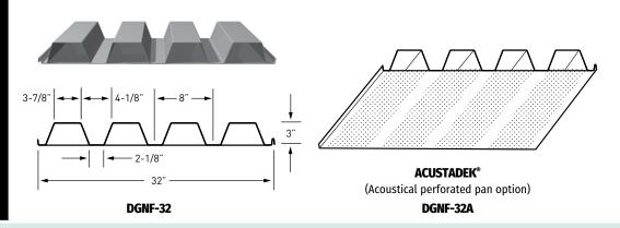
DGNF-32 provides designers section properties and diaphragm shear values for a variety of structural roof applications.
