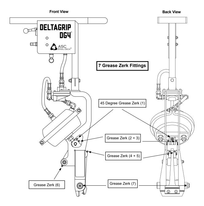
Please note that daily maintenance of this tool is required and is the responsibility of the tool user. Failure to do so can damage the shoulder screw, shackle pin, jaw, and frame. The renter of this tool (ASC Steel Deck Customer) will be responsible for all costs associated with the repair or replacement of damaged parts up to the value of complete tool replacement.
